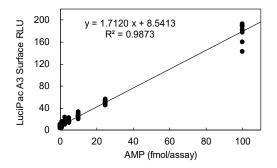
Table 2. Estimation of limit of detection (LOD) for adenosine triphosphate (ATP), adenosine diphosphate (ADP), and (C) adenosine monophosphate (AMP)from the data of pure analytes using LuciPac A3 Surface/Lumitester Smart system.
