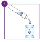
Transfer **3 drops (100 µl)** of the sample supernatant into the dilution tube by squeezing the extraction tube.
