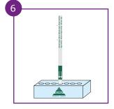
Once the liquid has flowed up to the wick pad, remove the test strip from the dilution tube and place it upright (arrows pointing down) into a slot of the vial rack. Allow the strip develop for **10 minutes** and read the result immediately.
