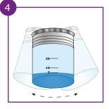
Transfer dilution buffer (bottle B) into the dilution tube up to one of the cutoff level marks (5/10/20 ppm gluten). Close the dilution tube with the cap and shake vigorously by hand for **15 seconds**.
