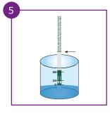
Take off cap and place a test strip vertically (arrows pointing down) into the dilution tube. Allow the liquid to flow up the strip to the wick pad (see arrow on the image). This takes about 45 seconds.
