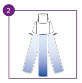
Close the tube with the cap and shake vigorously by hand for **1 minute**. Remove the cap from the extraction tube and replace it with a fresh dropper tip.
