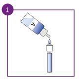
Add **0.2 mL** rinse water or weigh in **0.2 g** of homogenized sample into the extraction tube. You can estimate this amount by filling up one extraction tube cap. Fill tube with extraction buffer (bottle A) to the level shown in picture.
